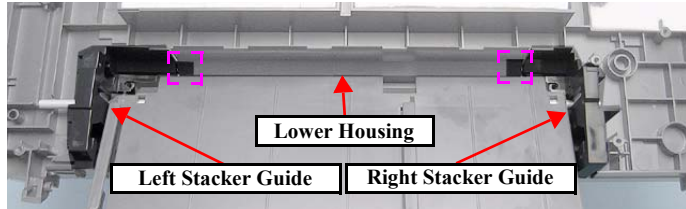
Figure 4-114. Reinstalling the Stacker Assy
