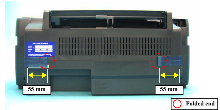
Figure 4-3. Securing the Middle Housing on its rear
